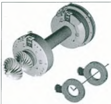
FIGURE 1. Electromagnetic cushions continually change in field strength to keep the rotor shaft centrally positioned.
